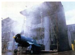
Figure 14: Weather testing at Cupples' plant in St. Louis Source: Lambot
